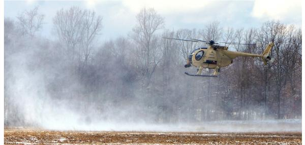
Fig. 1: Automatic landing of the Unmanned Little Bird.
