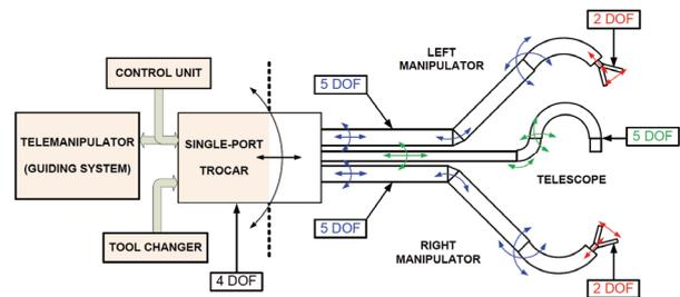
Fig. 1: Schematically design of the “Highly Versatile Single Port System”
