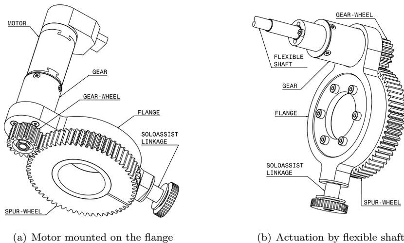
**Figure 4.14:** Concepts of the rotation for the single-port platform: a) Direct drive by attaching the motor on the flange b) Actuation at the periphery by using a flexible shaft
