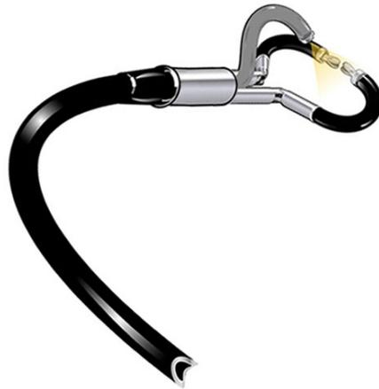
**Figure 7.1:** Schematic drawing of a fully flexible single-port platform for transluminal surgery.
