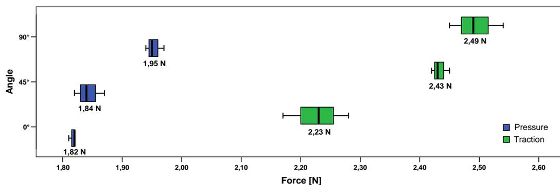
**Figure 6.11:** Results of the force measurements by vertical deflection of the bending section
