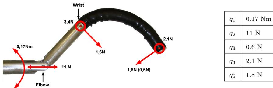
**Figure 6.14:** Applicable average forces on the single-port manipulator
