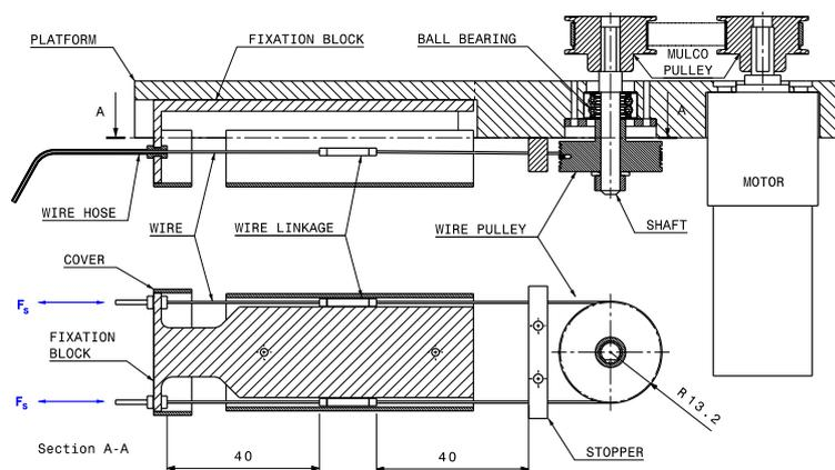
(a) Sectional view of the linear actuation mechanism
