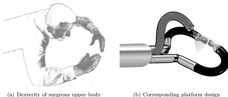
**Figure 3.3:** Design of a platform that emulates the skills of the surgeons, as if his upper body could be introduced through a small incision into the abdominal cavity.
