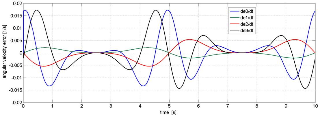
**Figure 5.6:** Error plot of the angular velocity of the tool tip in quaternions.
