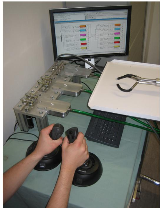
(b) Control of the manipulators with two joysticks
