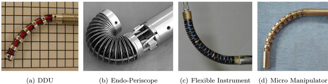
**Figure 2.2:** Instruments with flexible bending segments: a) Snake-Like Distal Dexterity Unit (DDU) [66] b) Endo-Periscope [75] c) Flexible Instrument Tip [65] d) Bending Micro Manipulators [61]
