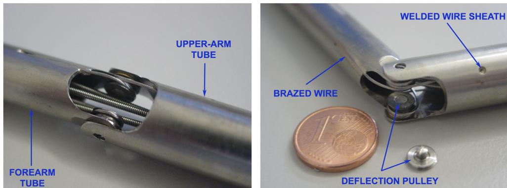
**Figure 4.5:** Elbow articulation of the single-port manipulator.
