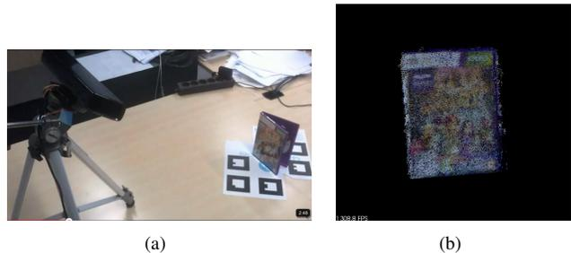
Fig. 1. Object recording setup (a) and merged point cloud (b)
