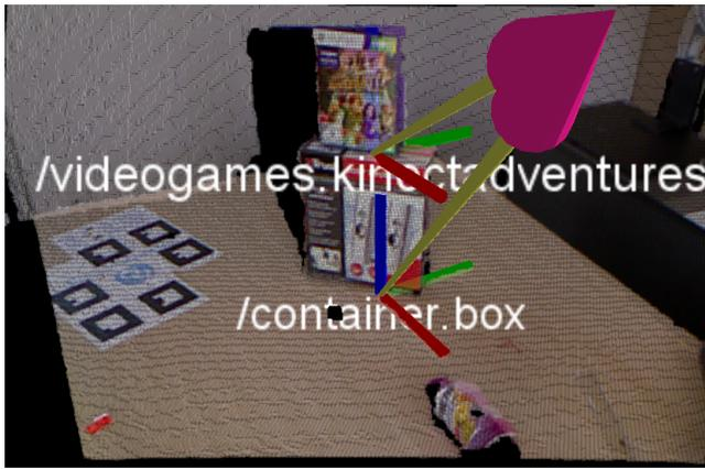
Fig. 2. Pose estimation using a Kinect camera and the method presented in section IV-B. The arrows indicate the position of the camera. The marker pattern is visible on the left.
