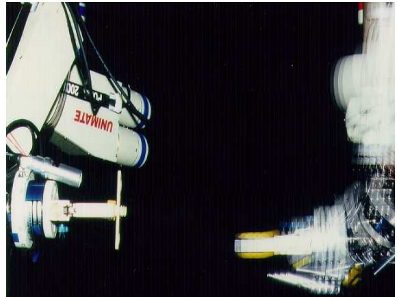
Figure 5: Robot 1 holding screw in hole, robot 2 holding cube and approaching.
