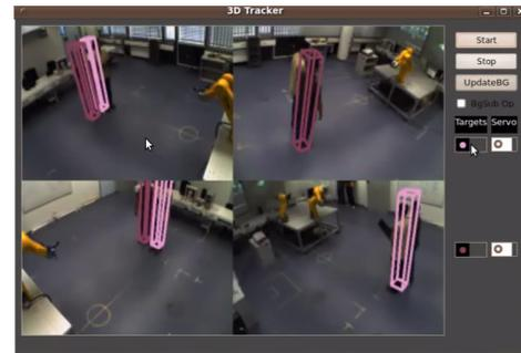
Fig. 11. The figure illustrates how the system detects occlusion between targets.
