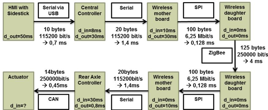
Fig. 4: Timings for the transmission of commands from the sidestick to the eCorner.  $d_{in}$  and  $d_{out}$  refer to the periodicity of the tasks processing the incoming and outgoing buffers, respectively.
