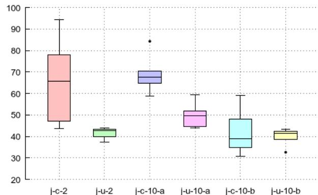
Fig. 7: Detailed results for the acceptance rates in different scenarios.  $j$ =jammer active;  $c$ =end of beam covered;  $u$ =end of beam uncovered;  $2$ =distance of 2m;  $10$ =distance of 10cm;  $a, b$ =different positions of wireless nodes; the results are given as percentages.
