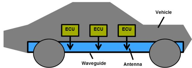
Fig. 5: Utilizing compartments of the vehicle as waveguides.
