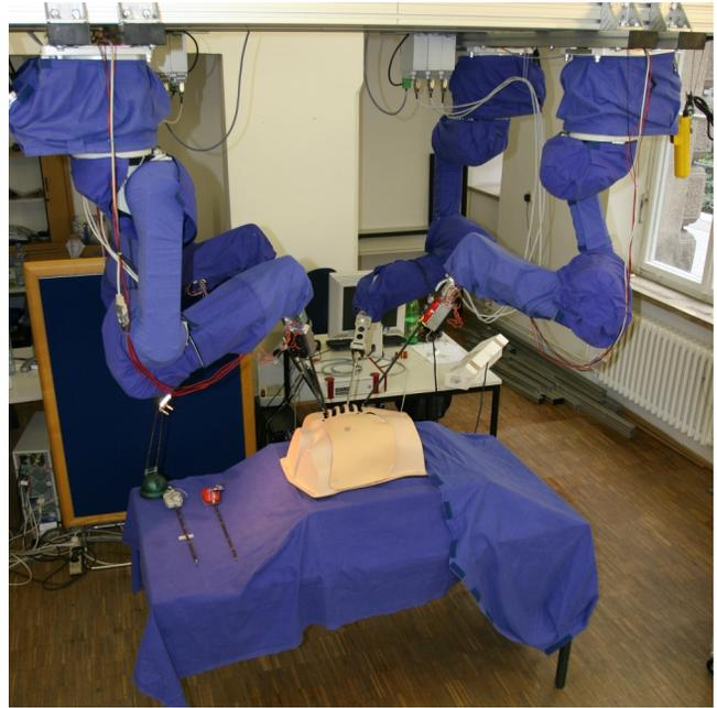
Fig. 1. **Hardware Setup:** Four ceiling mounted robots can be equipped with either a stereoscopic endoscope or different surgical instruments. Instruments are augmented with force sensors. In-output is accomplished at a master console, comprising two 6DoF force feedback devices.
