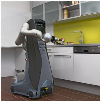
Fig. 9. Our mobile robot platform performing daily tasks, such as localization, objects detection, grasping and so on. Equipped sensors: three laser scanners, a Kinect camera and a stereo camera system.
