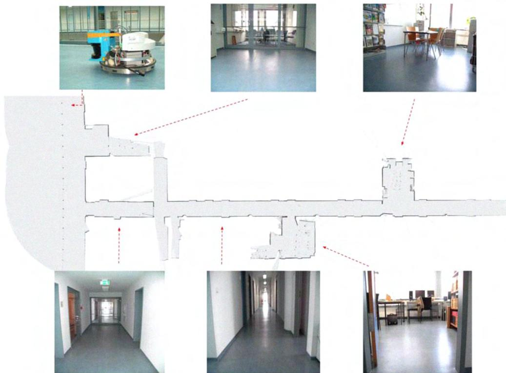
Figure 10: The automatically generated map of the Department of Informatics: Robotics & Embedded Systems at the Technische Universität München.
