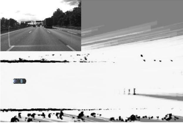
Fig. 10. Example for an occupancy grid in a freeway scenario. The left and right road boundaries are clearly visible.
