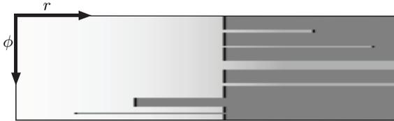
Fig. 3. Polar grid computed on the GPU with 70 simulated distance measurements and a depth resolution of 256 cells.
