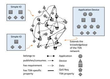
Fig. 1. Network Devices are analyzed by the application management service and the obtained new knowledge extends relevant parts (application, data, device, QoS requirement, device TSN-specific property) of the TSN network knowledgebase.
