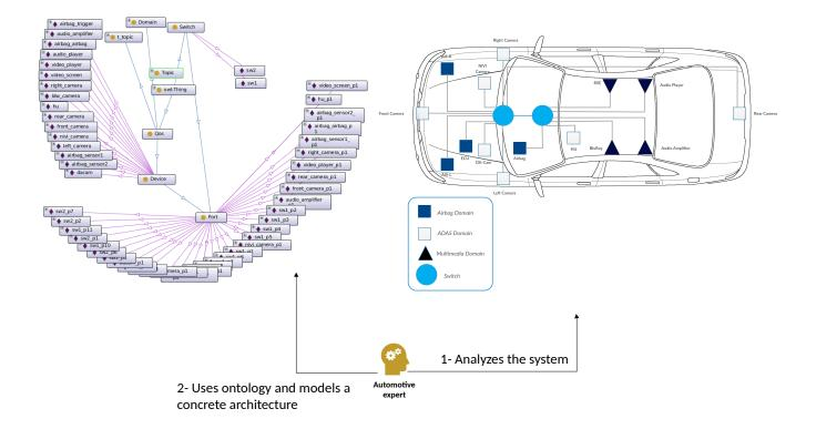
Fig. 10. This example shows how to use ontology classes and object properties to generate instances (individuals). An ADAS TSN network (right) introduced by [23] which is slightly changed with and airbag domain added into and analyzed using the ontology.
