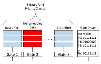
Fig. 8. TAS architecture contains 8 gates for 8 priority classes on each port. The Gate Driver decides which port has to be opened or closed based on a predefined event list. For example, at T1, only Gate 2 is open for transmission of high-priority data (Ethernet frames) without any interruptions by low-priority best effort data.
