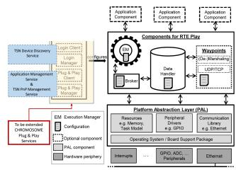
Fig. 4. CHROMOSOME architecture with its components and to be extended Plug-and-Play features. Figure is adapted from Buckel et al. [20]
