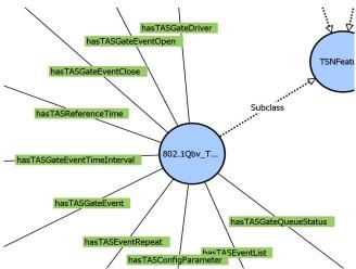
Fig. 9. Ontology data properties are used to model the properties of TAS. They build the most important knowledge for automatic configuration of TAS. An excerpt of the model is presented here.
