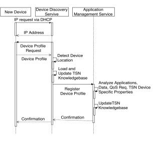
Fig. 2. Sequence diagram of the Plug Phase
