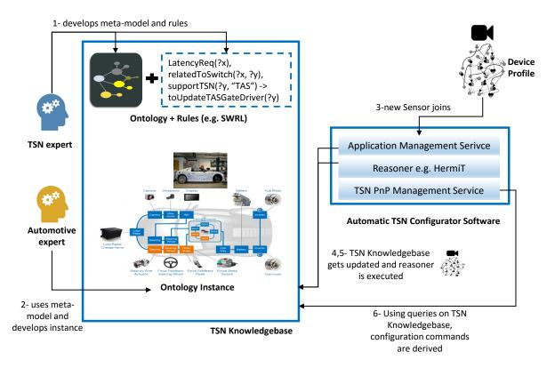
Fig. 5. Ontology-based approach for automatic TSN configuration. The figure uses RACE [22] in-vehicle communication architecture as an example that can be an use case of the developed approach in this paper.
