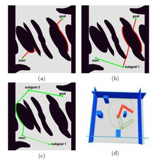
Figure 3: An example for the planning process in a static two dimensional environment shown in (d). In the cspace map in (a) the failure of the local planner starting from start and from goal can be seen. In (b) a first subgoal is tested that can be reached from the start but fails to be connected with the goal. In (c) the second subgoal tried leads to a solution. The planned path is shown in (d) as the movement of the tool center point.
