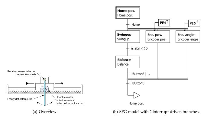
Figure 1: Experimental setup: inverted pendulum
