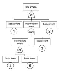
Fig. 10.4. A Fault Tree
