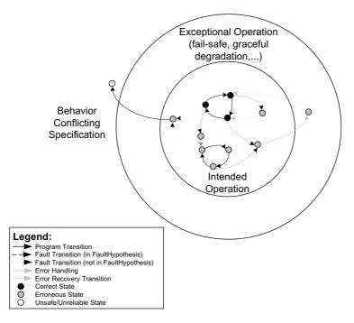
Fig. 10.2. Fault-Tolerance Concepts
