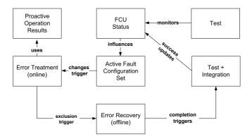
Fig. 10.8. Concept of Fault-Tolerance Mechanism
