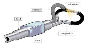
Fig. 1 Schematically drawing of the "Highly Versatile Single Port System"
