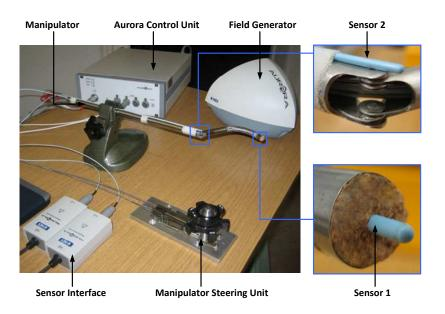
Figure 6.1: Electromagnetic tracking set-up for the workspace measurements.
