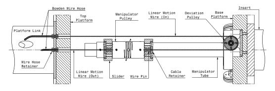
Figure 4.13: Sectional view illustrating the linear actuation mechanism of the manipulator
