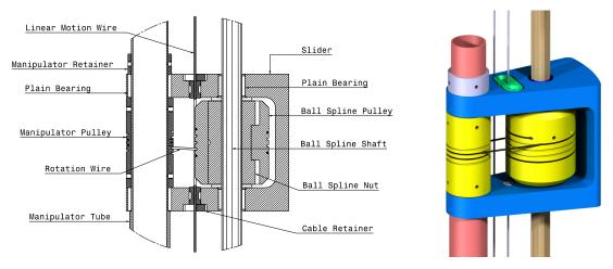
(a) Sectional view of the slider and the rotary mechanism
