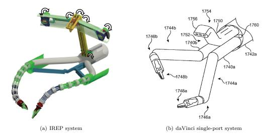
**Figure 2.3:** a) Insertable Robotic Effector Platform (IREP) for Single-Port Access (SPA) Surgery [68] b) Concept of the daVinci single-port system as claimed in the patent [106] (Intuitive Surgical, USA)
