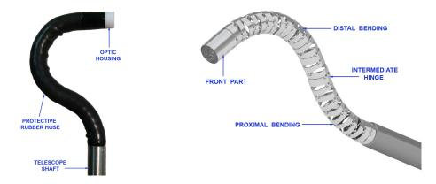
Figure 4.6: Double-bending telescope comprising two bendable sections and 3 DOFs in total.
