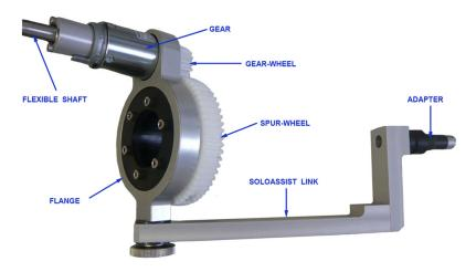
Figure 4.15: Rotary drive unit of the single-port platform attached to the SoloAssist link.
