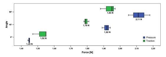
Figure 6.10: Results of the force measurements by horizontal deflection of the bending section
