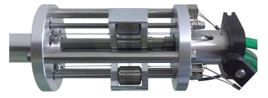
Figure 4.9: Proximal unit of the developed single-port platform including the linear and rotary articulations as well as the linkage for the guiding system.
