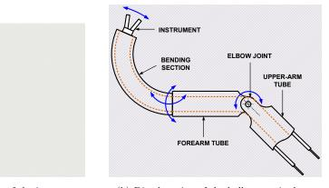
(a) Cross-section of the insert (b) Distal section of the hollow manipulator
