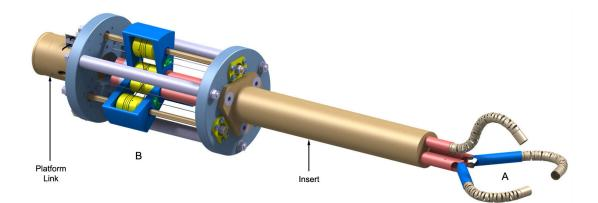
Figure 4.1: Design of the highly versatile single-port platform. A: Distal dexterity inside the body.
