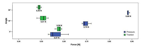
Figure 6.12: Results of the horizontal force measurements by bending the elbow joint
