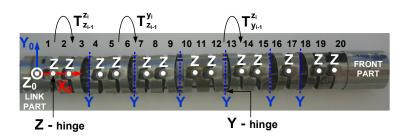
Figure 5.2: Bending section of the Karl-Storz gastroscope illustrating the configuration of the hinges and their orientations. The bending section comprises the three different "passive" joints Tzz, Tyz and Tzy.
