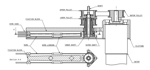
Figure 4.18: Sectional view of the drive unit and bowden wire mechanism for distal articulations
