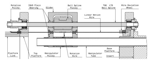
Figure 4.10: Sectional view of the linear and rotary actuation mechanism of one manipulator.
