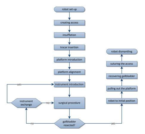
Figure 3.5: Surgical procedure of the single-port robotic gallbladder resection.
