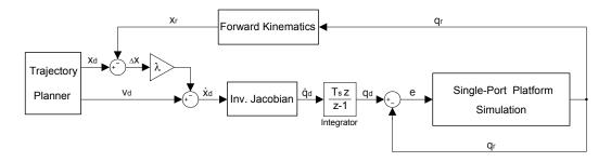
Figure 5.8: Velocity-based control of the single-port manipulator. A basic velocity profile is used to control the simulation of the platform.
