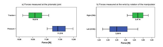
Figure 6.13: Results of the measured forces with the prismatic and rotational joints
