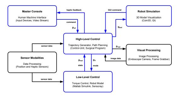
Figure 5.1: Concept of the control architecture for the single-port system. The high-level control forms the central control unit for all the modules. The provided and required interfaces  $p_{ref}$ ,  $p_d$  and  $p_{real}$  are the reference, desired and real tool positions.
