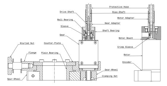
Figure 4.16: Sectional view of the rotary drive mechanism including the coupling of the shaft.
