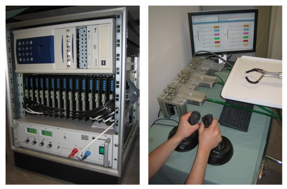
(a) Control hardware integrated in a 19-inch rack
