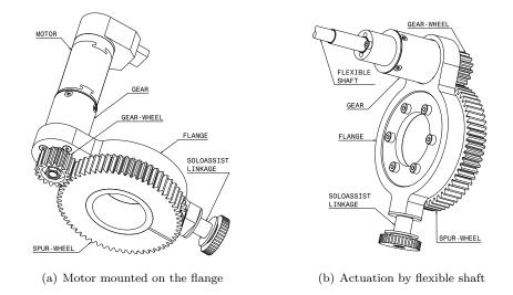
**Figure 4.14:** Concepts of the rotation for the single-port platform: a) Direct drive by attaching the motor on the flange b) Actuation at the periphery by using a flexible shaft
