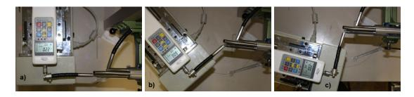
Figure 6.8: Measurement of the forces applied by the elbow joint on the manipulator tip at different bending angles of the elbow joint: a) straight configuration b) elbow bent to  $50^{\circ}$  c) elbow bent to  $80^{\circ}$
