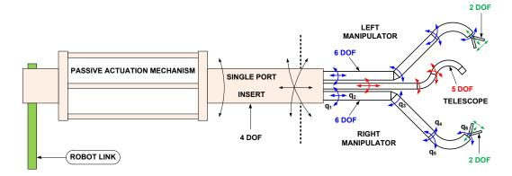
Figure 3.6: Schematic drawing of the semi-rigid single-port surgical platform: Two 6 DOF manipulators ( $\emptyset$ 12mm), a 5 DOF flexible telescope ( $\emptyset$ 10mm) and a 4 DOF robot guiding the insert ( $\emptyset$ 34mm).
