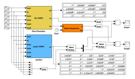
Figure 5.4: Matlab-Simulik program for the numeric verification of the Jacobian. DK\_HVSPS computes the forward kinematics and Jacobi\_HVSPS the Jacobian of the manipulator. In MatrixToQuaterenion, the quaternions q and the matrix  $M_q$  are determined from the rotation matrix  $R_e$
