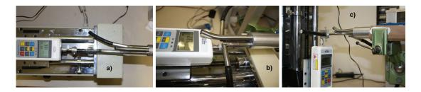
Figure 6.9: Linear force measurement of the prismatic joint and torque measurement of the rotational joint: a) pulling in straight form b) pushing with the upper-arm tube c) rotation force at the wrist
