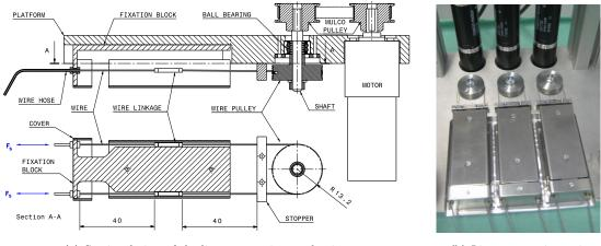
(a) Sectional view of the linear actuation mechanism
