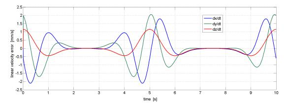
Figure 5.5: Error plot of the linear velocity of the tool tip.
