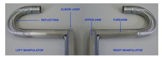
Figure 4.3: Distal section of the two single-port manipulators in opposed configuration.
