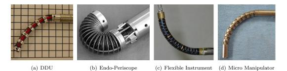
**Figure 2.2:** Instruments with flexible bending segments: a) Snake-Like Distal Dexterity Unit (DDU) [66] b) Endo-Periscope [75] c) Flexible Instrument Tip [65] d) Bending Micro Manipulators [61]
