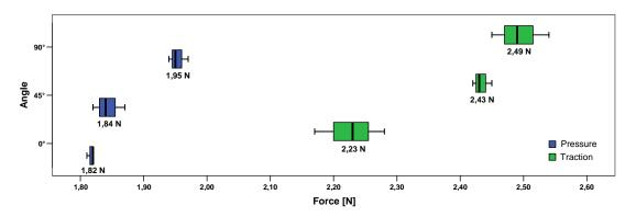
Figure 6.11: Results of the force measurements by vertical deflection of the bending section
