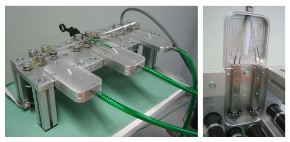
(a) Actuation unit for the deflecting and elbow joint of the manipulators
