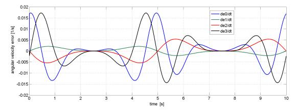
Figure 5.6: Error plot of the angular velocity of the tool tip in quaternions.
