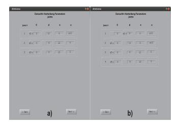
Fig. 5. Denavit-Hartenberg parameters of each Link. a) The parameters of robot in Figure 3 are presented, b) Parameters of the same robot with the extra dof. The number of rows and the column of the joint position variable are automatically defined by the toolbox
