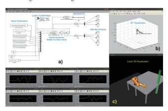
Fig. 7. Automatically generated Simulink block model. It consists of (a) the block model of the robot, (b) RT robot visualization and c) Coach 3D visualization. The user can modify the parameters of the robot and observe the different robot dynamic behaviors.
