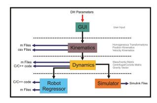
Fig. 1. Structure of the Robot Modeling/Simulation Toolbox.
