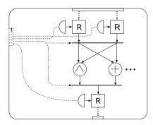
Figure 3. The final result for alu.action after flattening and optimizations.
