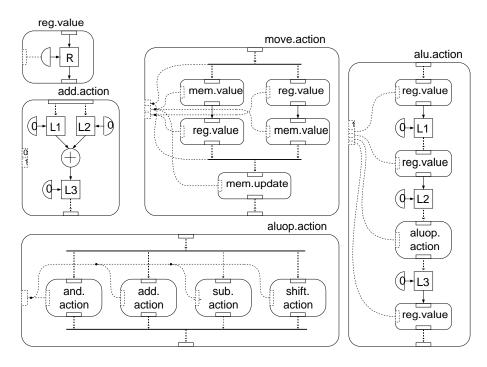
Figure 2. The image interfaces are represented by the ports at the left of each HMC feeding (dashed line) constant generators (drawn as half-circles), referenced HMCs or demultiplexer/multiplexer pairs.
