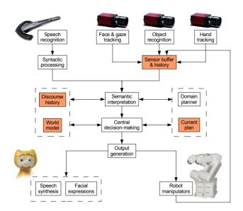
Figure 4: JAST system architecture
