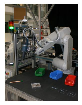
Fig. 5. Hybrid assembly station: tool station, robot arm (with electric drill) and assembly-table.
