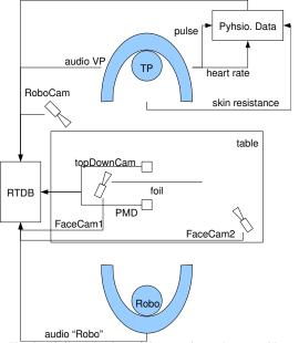
Fig. 2. Schematic view of the experimental setup with sensors.
