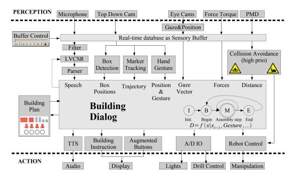
Fig. 4. Functional system overview with perception, cognition and output based on the RTDB.
