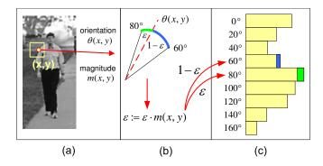
Fig. 2. Feature extraction as it is done for each pixel (x,y) inside a cell/block: (a) computation of gradient orientation and magnitude (b) orientation interpolation and weighting (c) vote binning for the used directions.
