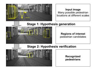
Fig. 1. Two-staged recognition process of our system.
