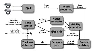
Fig. 3. Flow of the visual tracking system
