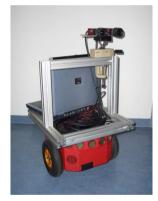
Fig. 8. The Pioneer3-DX carrying the two Marlin cameras.
