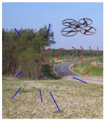
Fig. 1. The  $Z_{\infty}$  algorithm estimates the rotation (red) and the translation up to scale (blue) based on a monocular camera in an efficient way. Therefore, it fits well for resource-limited systems like e.g. flying mobile robots.
