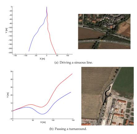
Fig. 17. Two trajectories measured by the  $Z_{\infty}$  algorithm (red) and the IMU (blue). In the pictures at the right-hand side the driven trajectories are sketched in black.
