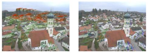
Fig. 20. Motion estimation based on SURF features.
