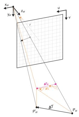
Fig. 3. This drawing visualizes how the measurable translational component  $\Delta T_x$  can be calculated. In general the optical flow vectors become longer the more parallel they become to the image plane and the closer they get to the image border. The orange auxiliary line illustrates the projections onto the x-z plane.
