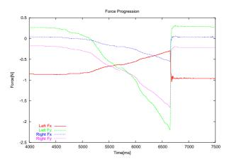
Figure 8. Breaking Ethicon 7/0 during knot tying
