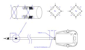
Figure 2. APPLICATION OF STRAIN GAUGES TO AN INSTRUMENT
