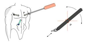
Figure 3. TROCAR POINT KINEMATICS
