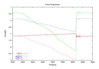
Figure 7. Breaking Ethicon 7/0 by normal pulling
