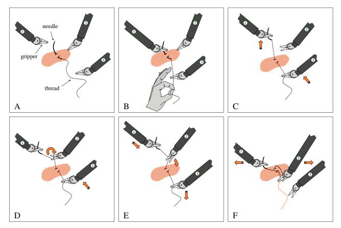
Fig. 3. **Minimally invasive knot-tying**. (A) The knot-typing procedure starts with the needle and three grippers in this configuration. (B) Gripper 1 takes the needle, and the thread is fed manually to gripper 3. (C) The thread is pulled through the puncture, and (D) wound around gripper 2. (E) Gripper 2 grabs the thread between the puncture and gripper 3. (F) The knot is finished by pulling the end of the thread through the loop.
