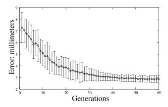
Fig. 6. **Evolino learning curve.** The plot shows the average error on the training set measured in millimeters for the best network in each generation, averaged over 50 runs. The vertical bars indicate one standard deviation from the average.
