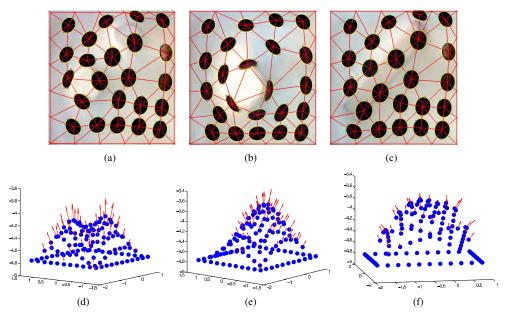
Fig. 7. 7(a),7(b),7(c) Illustrate the captured and processed images from the CCD camera for three different objects, and 7(d),7(f),7(f) the respective 3D reconstructions, and force distributions. Here the force vectors are illustrated with a minus sign, for visualization purposes.
