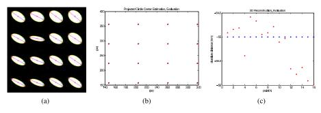
Fig. 6. 6(a) Illustrates the generated image that contains the projections of circles with known poses. In 6(b) are plotted the estimated (red) and known (blue) circle center projections, and correspondingly the absolute distances from the camera center are illustrated in 6(c).
