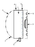
Fig. 1. (1): LED, (2): CCD camera, (3): a valve to regulate the amount of air within the frame, (4): rigid circle markers, (5): rubber skin surface, (6): the airtight frame of the finger,(7): glass, (8): air.
