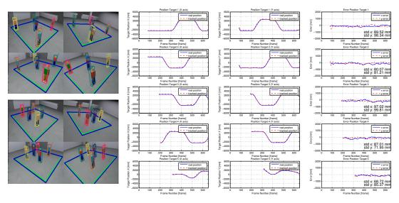
Figure 10: Illustration of the tracking system with 5 targets in the scene moving close to each other and two targets having similar appearance.
