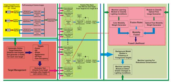
Figure 1: The figure illustrates the block diagram of the multiple human tracking system.
