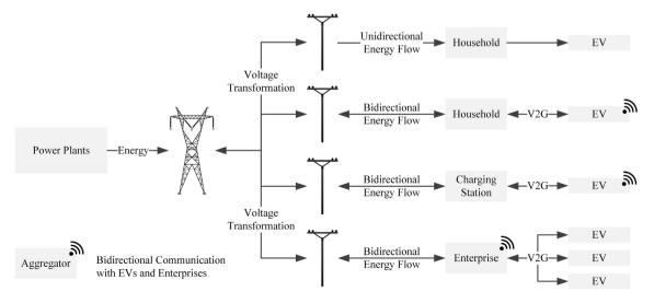
Fig. 1. The V2G concept: energy and communication flows. Adapted from Ref. [9].
