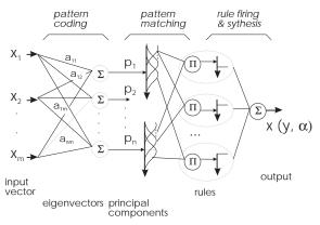
Figure 3: The task based mapping can be interpreted as a neuro-fuzzy model. The input vector consists of pixels of a grey-scale image.
