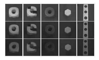
Figure 9: 15 grasping scenarios; from left to right: yellow cube, partly covered yellow cube, blue cube, yellow screw head, ledge with 3 holes; from top to bottom: optimal, worse and poor illumination.
