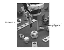
Figure 1: The end-effector of the manipulator with a handcamera (positioned optimally over the yellow cube).
