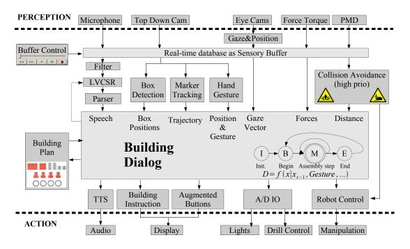
Fig. 5. Functional system overview with perception, cognition and output based on the RTDB.
