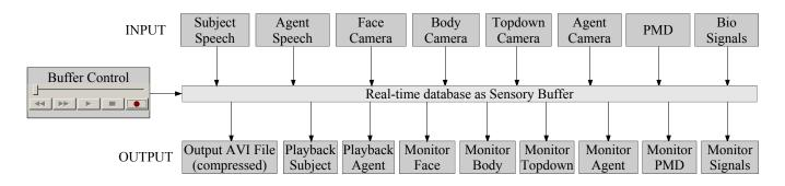
Fig. 1. Overview of the multi-modal recording scheme with the RTDB.
