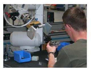
Fig. 6. Working cell with human worker and industrial robot arm.
