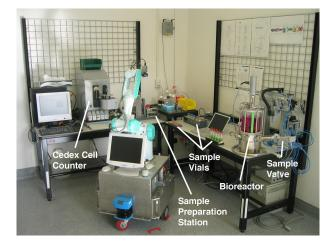
Figure 2: The robot lab for the cell counting sample management process with all necessary devices.
