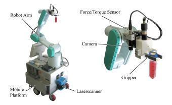
Figure 1: The mobile robot as it was shipped to the customer.
