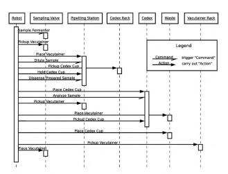
Figure 7: The implemented sample management process as an UML sequence diagram. The boxes on the top represent the devices, which the robot needs to operate. The two different kind of arrows symbolise commands, which are triggered by the robot and actions which the robot carries out itself.
