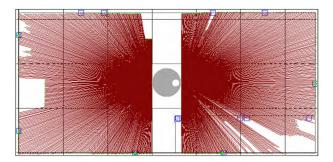
Figure 2: Localisation via the onboard Laser range finders.
