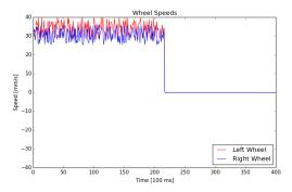
(b) Speeds of the left and right wheel at each time-step during the simulation. The speeds decrease to zero after collision.
