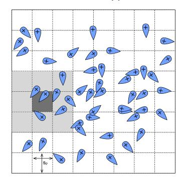
Fig. 3. Environment partitioned using perception range  $(s_p)$  information
