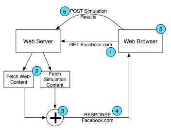
Fig. 2. The six stages of interaction and result calculation
