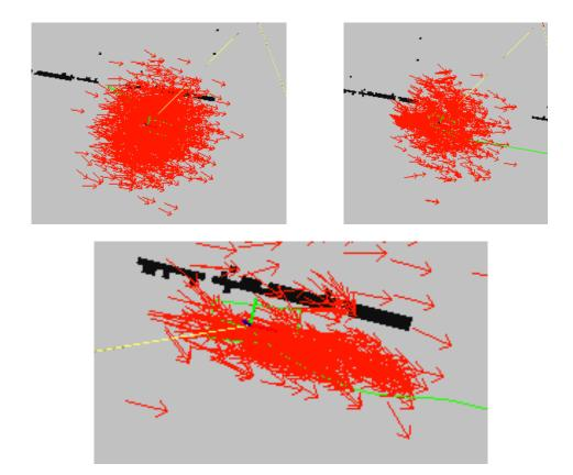
Figure 4.5: *Localization array*. The picture shows the step by step localization during the car's driving. At the beginning the estimation cloud is very big, but as soon as the car starts driving the estimation gets more precise.
