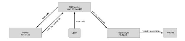
Figure 3.3: *Basic relation model of the hardware*. This graph shows the relation between the different hardware used for the car.
