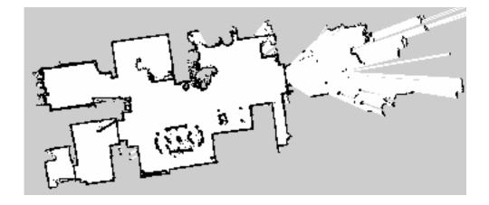
Figure 4.1: *SLAM map of a main floor*. The map shows the main floor of my home. The stripes on the right side of the picture shows perfectly the problem of a glass door as obstacle.
