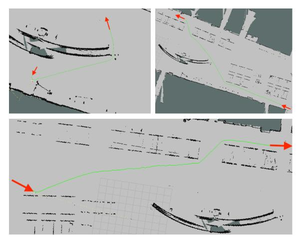
Figure 4.3: *Global routes*. Here are some global routes presented. The green lines are the calculated routes from the estimated starting point (arrows with peak to the lines) to the set goal (arrows with peak away from the lines). The arrow peaks also show the front of the car at the beginning and the end.
