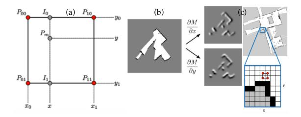
Figure 3.4: *Hector\_SLAM filter method.* "(a) Bilinear filtering of the occupancy grid map. Point P<sub>m</sub> is the point whose value shall be interpolated. (b) Occupancy grid map and spatial derivatives."[18] (c) A small zoom of the whole grid map.
