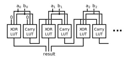
Figure 2.3.: A ripple-carry adder implemented using only 3-input LUTs
