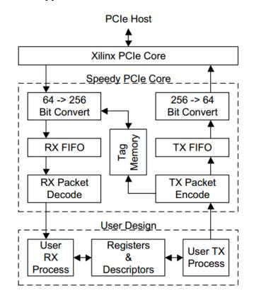
Figure 3.1.: Speedy PCIe IP core design (Image from [8])
