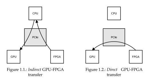
FPGA board shall communicate directly over the PCIe bus with minimal coordination by the CPU. A significant bandwidth improvement compared to the indirect method is to be expected.
