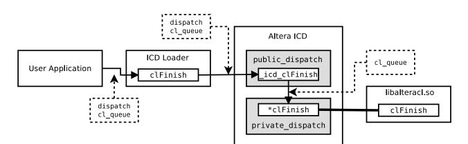
Figure 4.2.: Call graph for the function clFinish. The application calls the ICD loader function, which forwards the call to the wrapper function in the vendor ICD stored in the dispatch struct. The wrapper function then calls the real OpenCL function. The dashed boxes illustrate the contents of the arguments.
