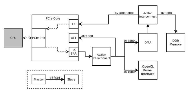
Figure 5.1.: Simplified configuration of the Altera OpenCL IP stack on the FPGA. Note that the solid arrows represent master/slave relationships and not necessarily the data flow direction.
