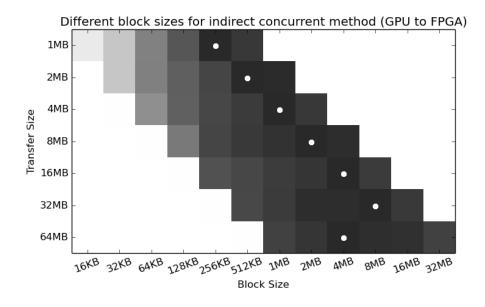
Figure 7.2.: Influence of the block size parameter on the performance for the concurrent indirect transfer method. Higher bandwidth is darker. The white dots mark the maximum bandwidth for each transfer.
