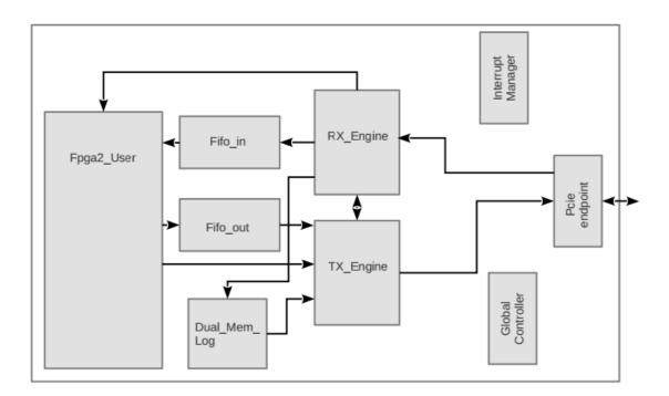
Figure 3.2.: FPGA<sup>2</sup> IP stack design (Image from [33])
