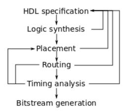
Figure 2.5.: The major phases involved in the configuration procedure. Falling back to a previous step may be required if a constraint cannot be met. (Image based on [17])
