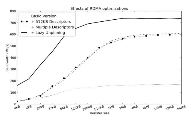
Figure 7.1.: Comparison of the optimizations described in section 5.3.2. Each optimization is added to the previous version (i.e. the Lazy Unpinning benchmark also includes the Multiple Descriptors and 512KB Descriptors optimizations). The Lazy Unpinning benchmark does not include the first transfer, which performs the actual memory pinning.
