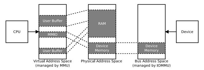
Figure 2.7.: Relationship between the different address spaces with example mappings. In this case the IOMMU performs a 1:1 mapping. (Image based on [32, 29])
