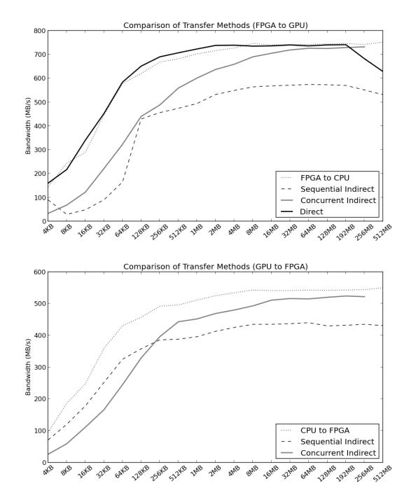
Figure 7.3.: Comparison of sequential indirect, concurrent indirect and direct transfer methods.
