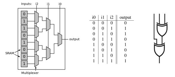
Figure 2.2.: Left: A look-up table loaded with the values of the 3-input XOR function which can also be seen as a 1-bit full adder without the carry output (Image based on [16]). Center: A truth table describing the same function. Right: An equivalent digital circuit consisting of logic gates.
