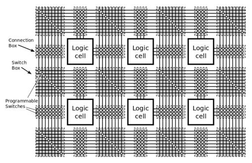
Figure 2.4.: Example of an island style connectivity (Components are not to scale. Image based on [17]
