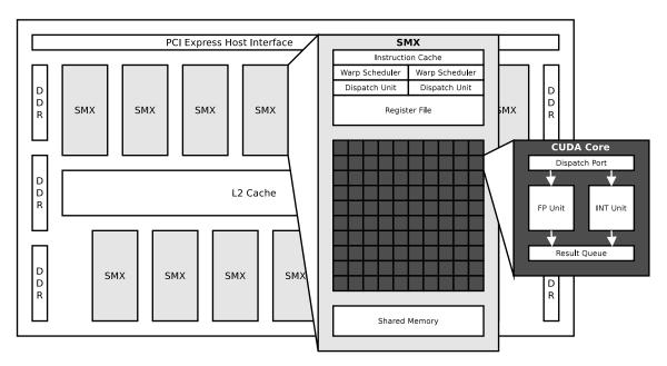
Figure 2.1.: Simplified schematic diagram of the NVIDIA GK110 class GPU architecture. (Image based on [13])
