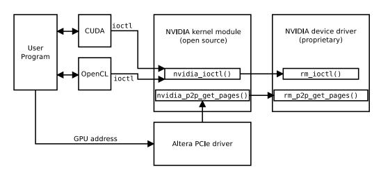
Figure 5.3.: Communication between CUDA/OpenCL and the NVIDIA driver
