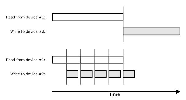
Figure 6.1.: Comparison of sequential (top) and concurrent (bottom) indirect transfer strategies. The two large transfers are splitted into 10 smaller transfers, 8 of them can be performed simultaneously. The gray vertical lines represent synchronization barriers.
