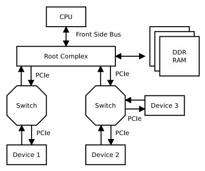
Figure 2.6.: Example topology of a system employing PCIe (Image based on [11])
