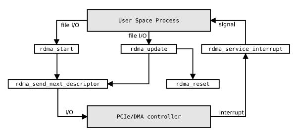
Figure 5.2.: The main functions of the new RDMA component
