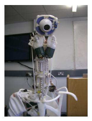
Figure 2: The prototype head and neck.
