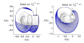
Fig. 5. Reachable set for the movement along the first arc. The curves represent exemplary trajectories starting in the set of initial states.
