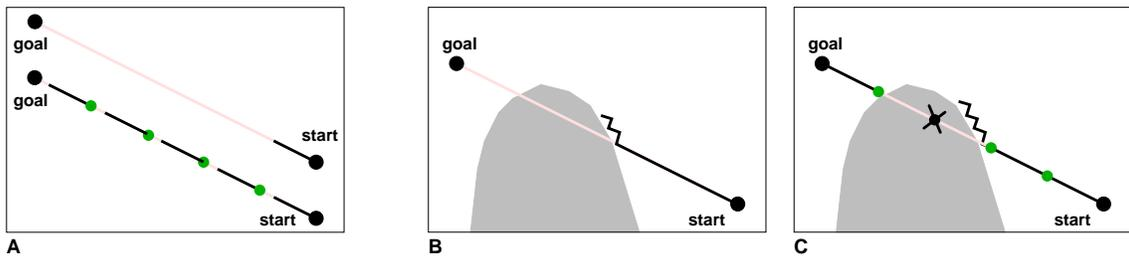
Figure 4: A: Parallel execution of straight line collision detection results in (almost) linear speedup. B and C: If there are obstacles along the straight line, some intersection points might not be accessible and the more expensive slide steps are not accelerated.
