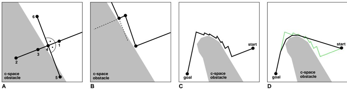
Figure 2: A: Local search for collision-avoiding positions to execute a slide step. B and C: Repeated slide steps can solve the planning locally. C: The path is smoothed through local optimization.
