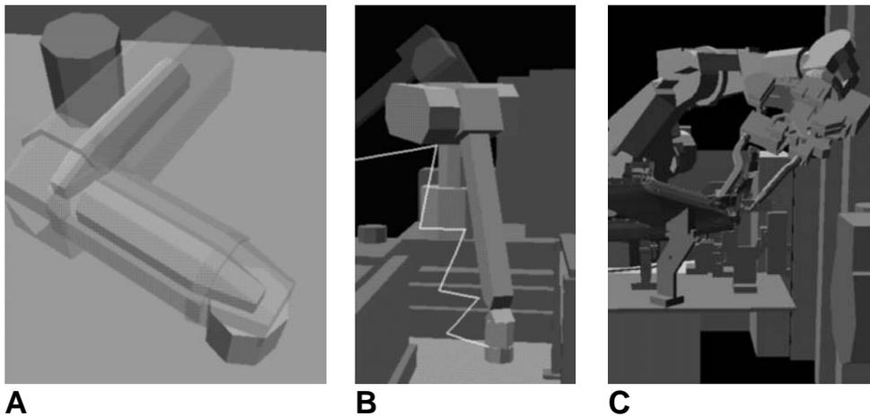
Figure 1: A: The geometry model is expanded to reduce the number of collision tests. B: An example of a path planned with slide steps in a 6 DOF environment. C: A very complex environment and robot model in an industrial environment.
