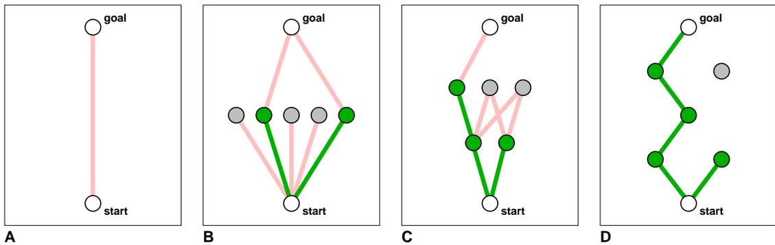
Figure 3: The global planner constructs a subgoal tree, growing from start into the set of random subgoals. Bright lines indicate failure, dark lines success of local planning.
