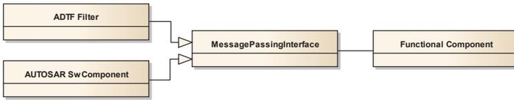
Figure 4: Excerpt of our implementation architecture for functional code and corresponding wrappers
