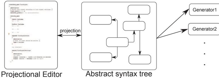
Figure 2: MPS projectional editing concept. The editor changes the AST directly. Generators build different representations of the model.
