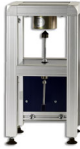
Fig. 5. Rod controlled by switched solenoids
