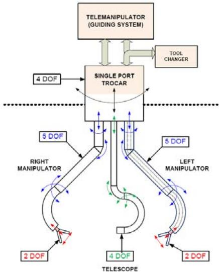
Figure 1: Schematically drawing of the "Highly Versatile Single Port System"
