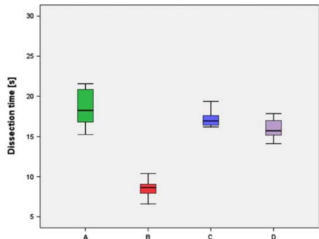
**Fig. 4** Comparison of the different ultrasonic dissectors in terms of speed in cutting a steak of beef 0.5 mm wide and 30 mm long ( $p = 0.001$ )
