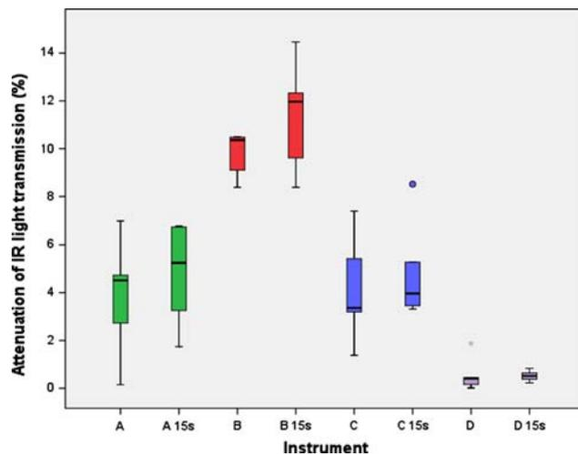
**Fig. 3** Light attenuation during dissection of lard. For each instrument, the percentage of attenuation both immediately after cutting and 15 s later without instrument activity was recorded ( $p < 0.001$ )
