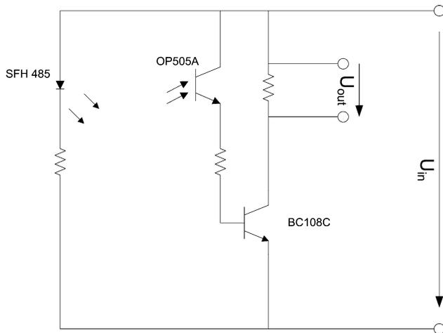
**Fig. 1** Circuit for measurement of light attenuation. On the left side, the light-emitting diode is powered. The central part is the light analysis part with signal amplification.  $U_{in}$  is the supply voltage, and  $U_{out}$  is the measured signal
