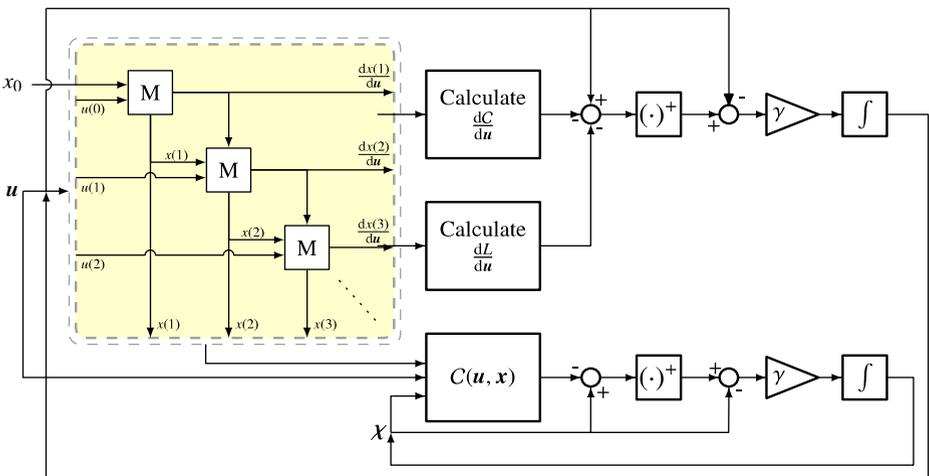
**Fig. 1** Block diagram of the controller. With the exception of the shaded block, the other operations can be run in parallel. Inside the shaded block a cascaded connection is used to calculate  $\frac{dx(i)}{du}$  from  $\frac{dx(i-1)}{du}$
