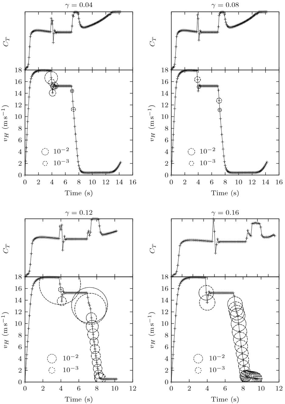
**Fig. 6** The variance of the neural network output with respect to time and helicopter sink rate for four values of the learning rate parameter. Larger circles mean larger variance while variances smaller than  $10^{-4}$  are not shown. For comparison purposes the thrust coefficient at the corresponding time is also provided
