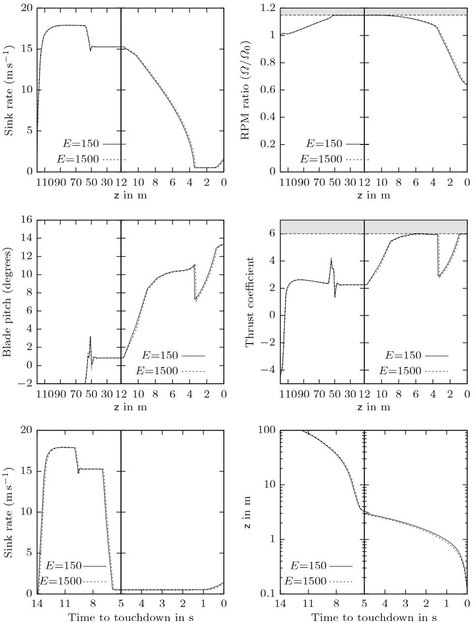
**Fig. 2** The sink rate, rotor rpm and control input of the OH-58A for a descent from an initial altitude of 120 m ( $N_s = 10$ ,  $N_c = 5$ ). The shaded regions represent the posed constraints. The scale on the right side of the graphs has been altered to show the last stage of the descent in higher detail
