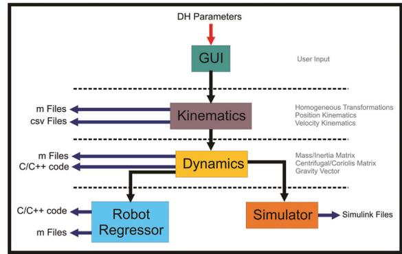
Fig. 1. Structure of the Robot Modeling/Simulation Toolbox.
