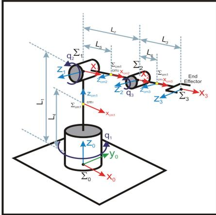
Fig. 3. Robot coordinate frames. The image shows 7 coordinate frames, 3 for each link, 3 for each center of mass and 1 for the robot base (reference frame),  $q_1$ ,  $q_2$  and  $q_3$  are the joint positions.
