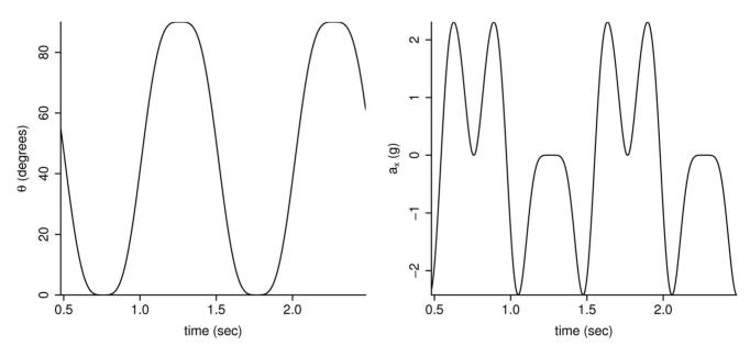
Figure 2. Robot joint angle and horizontal acceleration for condition: 1 Hz, amplitude  $45^{\circ}$ , radius = 0.5 m. doi:10.1371/journal.pone.0061691.g002
