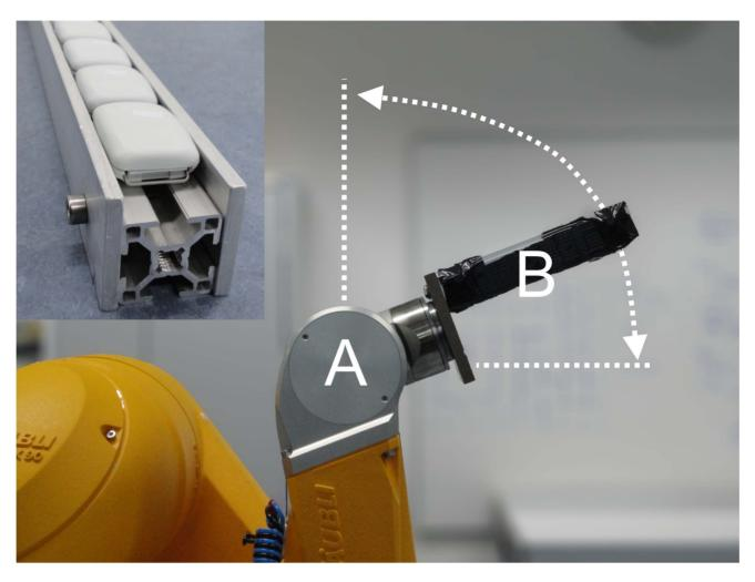
**Figure 1. Experimental setup.** A bar (B) holds five accelerometers and rotates around robot joint (A). doi:10.1371/journal.pone.0061691.g001
