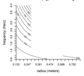
Figure 3. Robot conditions and corresponding reference acceleration (mg), where A = amplitude of angle. doi:10.1371/journal.pone.0061691.g003
