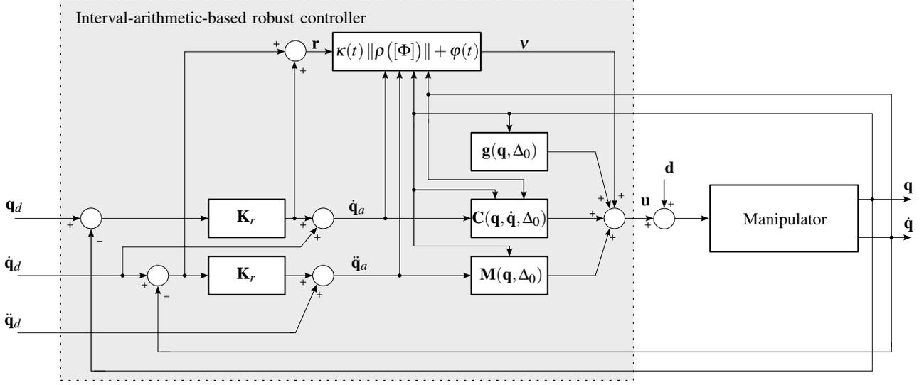
Figure 1. Block diagram of the closed-loop system.
