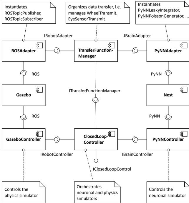
Figure 5 The components of the simulation backend in the NRP
