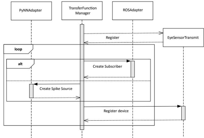
Figure 6 Transfer Function Initialization
