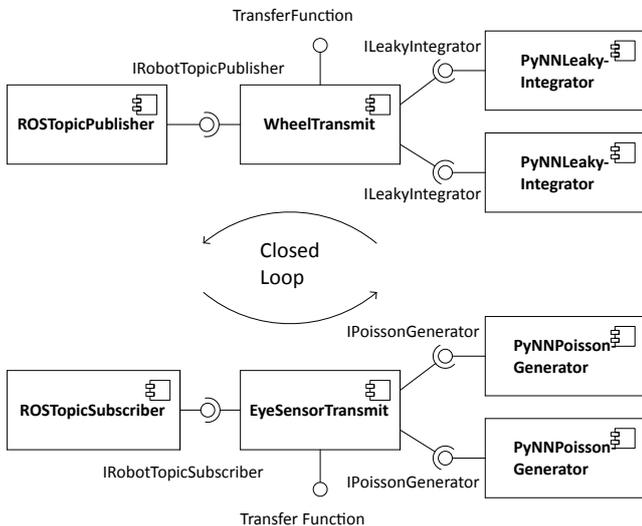
**Figure 4** Transfer Function components and their communication adapters in a running simulation of the standard image processing experiment
