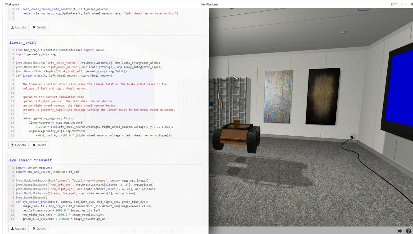
Figure 11 Editing Transfer Functions during a simulation
