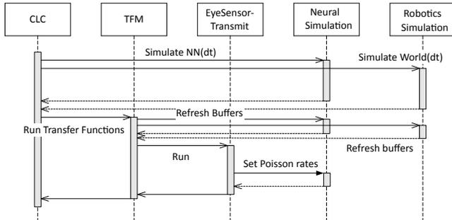
**Figure 7** Synchronization of simulations
