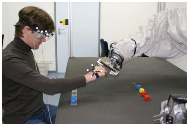
Fig. 5. Picture of the experimental JAST-Human handover setting.
